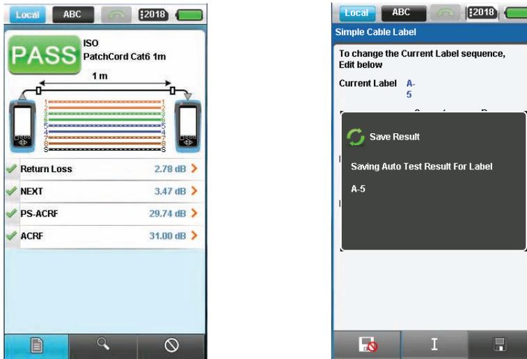
Once the test is complete, the reports can be exported using a USB flash drive and the results can be consolidated using the PC software ReportXpert. WireXpert provides a single page test report per patch cord providing both local and remote end results in a single page report.
