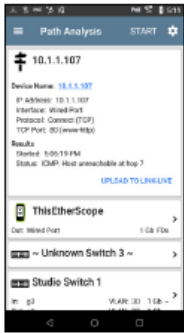
Path Analysis shows the device & interfaces that UDP/TCP traffic traverses
